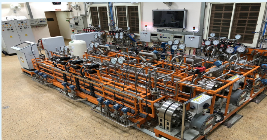
Supercritical carbon dioxide test loop at IISc (Photo courtesy: ICER)
