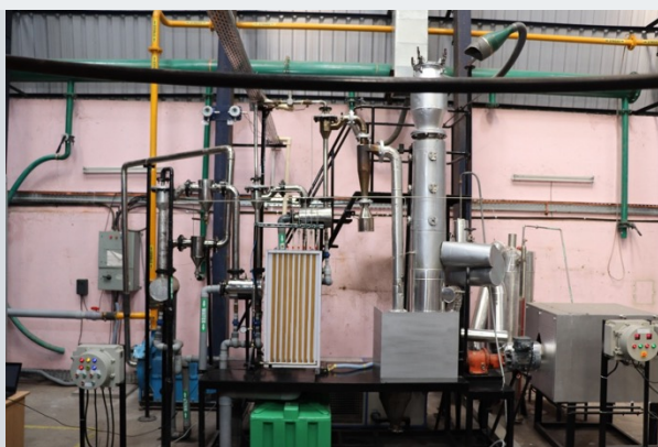
Biomass gasification unit with throughput of more than 0.7 kg per hour of ultra-pure green hydrogen (Photo courtesy: Dasappa S)
